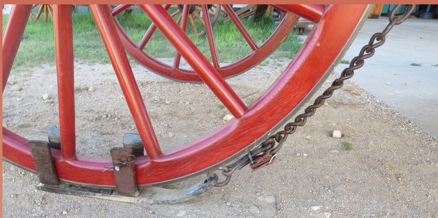
Figure 2: Modern rough lock in use, courtesy of Doug Hansen.
